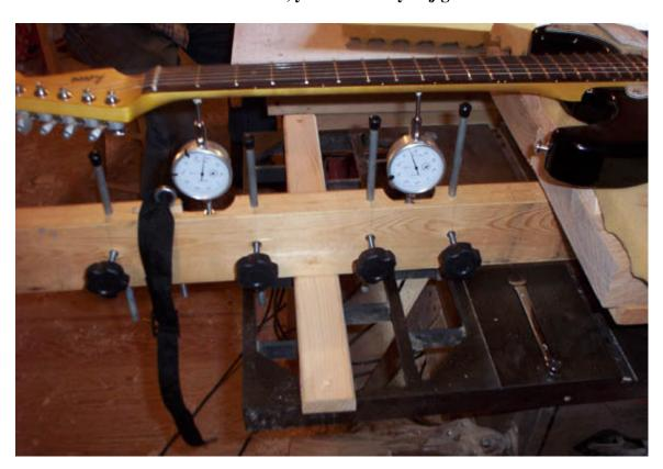
Don't worry about what the dial indicators read at this point; just make sure they are contacting the back of the neck though.
