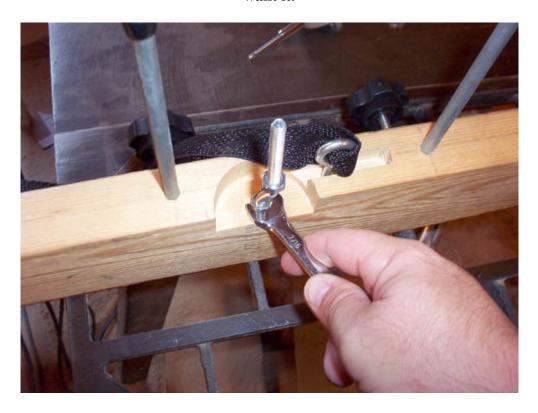
Now to hold the dial indictors in place all I did was use two 1/4" nuts on both sides of the mounting bracket to hold it wherever it needs to be. It's easy to move it up and down now by moving the nuts up or down. You'll have to experiment to get the proper placement depending on which guitar your jigging. It doesn't take long to figure out though, and making mental notes of where it was, for a particular style guitar, helps also.
