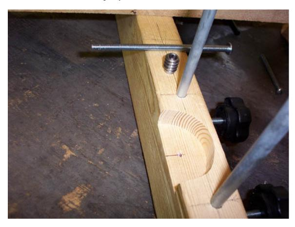
Now for the threaded inserts that I'm using it takes a 3/8" hole, so using the drill press again, I drilled a hole at least 2" deep just in case I later decide to use longer threaded rods. You'll probably have to move the support rods in order to use the drill press.
