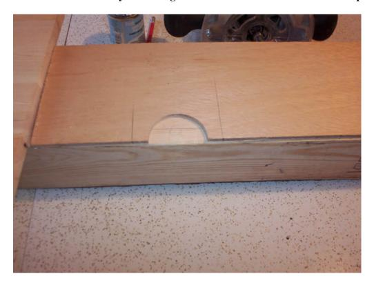
After the first dial indicator recess was routed out, I made a mark 3/4" away from the 3rd hole from the board and placed the dial indicator recess jig so that the left edge of the circle touched it. Double stick taped it down again with another 2x4 past it to hold the template flat and routed out the second recess.
