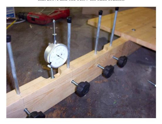
Here's another angle of the dial indicator. It looks tilted to the left, but that's because of the way the picture was taken. The main object is to make sure that the dial indicators are in line with the support rods.
