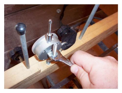
After both the dial indictors have been tightened into place it was time to move on to the mini jack. For right now I just used a cork circle and glued it to the top to protect the headstock. You can use whatever you feel is safe though.
